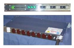
The 51133 series is a three phase 19" rack mount power distribution unit that is 1 "u" (1 ¾") high and 9" deep. This series has nine IEC320 C13 receptacles on the rear. This series comes standard with a branch rated circuit breaker. Standard options like remote control, filtering, and other options are available. The 51133 series comes in various current ratings depending on model, see the specs below.
