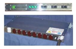
The 51132 series is a three phase 19" rack mount power distribution unit that is 1 "u" (1 ¾") high and 9" deep. This series has eight NEMA 5-20R receptacles on the rear. This series comes standard with a branch rated circuit breaker. Standard options like remote control, filtering, and other options are available. The 51102 series comes in various current ratings depending on model, see the specs below.
